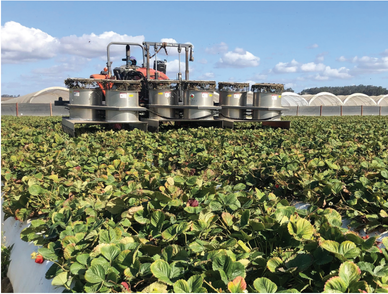
Figure 13. A recently optimized tractor-mounted bug vacuum improved the efficacy of removing Lygus bugs by 2.2 times over the previous version (Wells et al., 2020).
